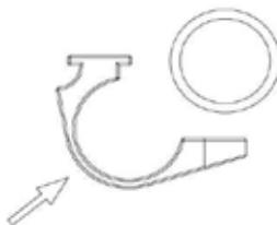
Step2: make the instrument slip insert the snap ring from right to left.
